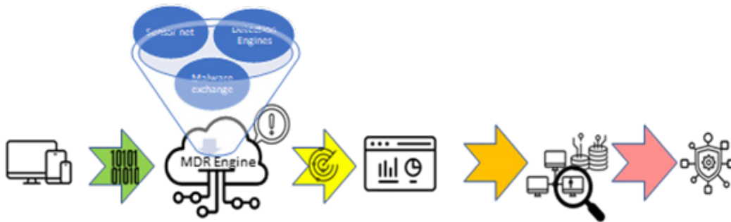
Figure 1: Sources forward logs to the managed detection and response (MDR) engine, which uses Proofpoint threat intelligence to create enhanced alerts. Our team triages, analyses and prioritises the alerts, then it conducts correlational analyses and proactively hunts threats to contain and respond to them.
